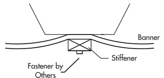
Stiffeners are attached at both ends. An intermediate stiffener is attached at the mid-point of Banners longer than 120". Intermediate stiffeners are shipped loose and attached in the field.
